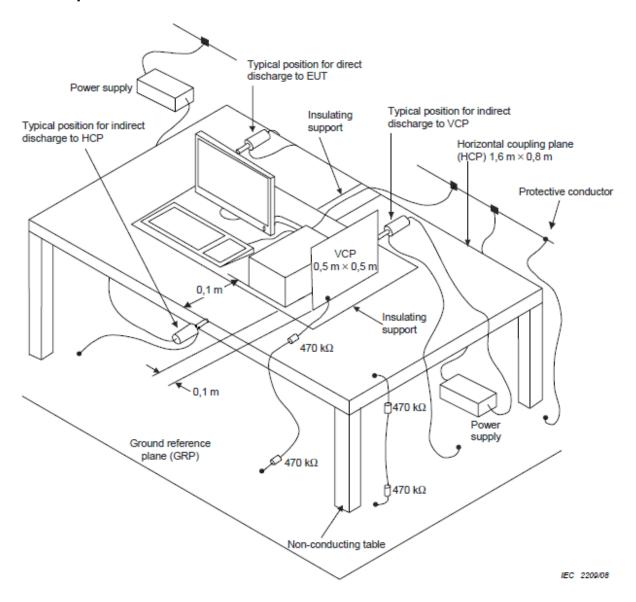
The test setup consists of the test generator, EUT and auxiliary instrumentation necessary to perform DIRECT and INDIRECT application of discharges to the EUT as applicable, in the follow manner:
