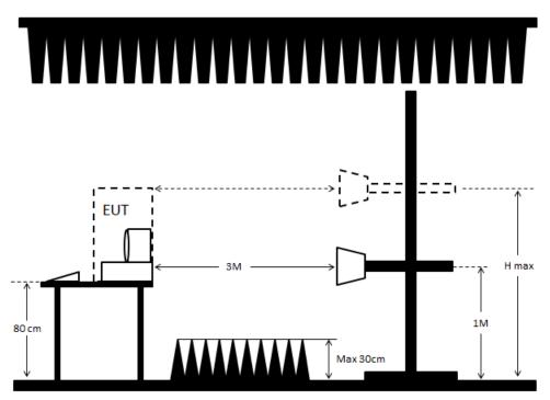
Remark: When EUT height is over 172cm, H max = Top of EUT
