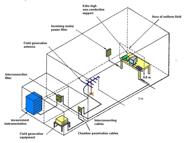
The procedure defined in this part requires the generation of electromagnetic fields within which the test sample is placed and its operation observed. To generate fields that are useful for simulation of actual (field) conditions may require significant antenna drive power and the resultant high field strength levels.
